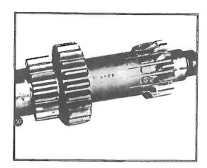
Gear teeth chipped and broken away from the engaging ends of the teeth indicate partial engagement and dragging clutch, which keeps the countershaft turning so that there is interference with gear engagement.
