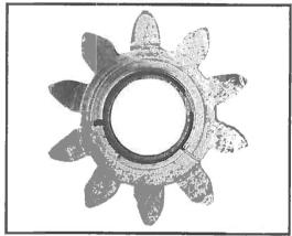
A fatigue crack extending from the root fillet to the bore.
