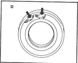
This bearing was dropped. It landed so that the cage was bent at the large end. This cage distortion causes the roller to bind in the cage and distort.
