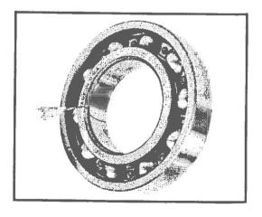
There are three types of damage resulting from improper installation. The first is a split race caused by forcing the bearing onto a shaft too large for the inside diameter of the bearing race.
