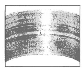
These show when a particle of dirt was left during bearing installation; it caused damage by pushing the bearing inward increasing localized pressure and heat.
