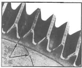
Fractures caused by repeated, heavy loads on several teeth of a spur gear are shown. The tooth marked "A" apparently broke first (note smooth velvety zone) as a result of a fatigue crack.
