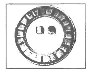
The first indications of fatigue failure may be noisy running and increased vibration. The bearing races show the metal surfaces of the races have flaked away. This flaking is caused by the effects of excessive speed and load.
