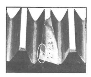
This shows fatigue at the root of three pinion teeth.
