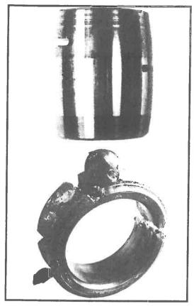
The broken cage was caused by intermittent lack of lubricant. At times, because of certain operation conditions, the oil fails to get to the bearing for a period long enough to cause light scoring of rollers and rib. This causes pressure on sides of cage pockets. After this has repeated a number of times, the cage finally starts to crack and then break up as shown.
