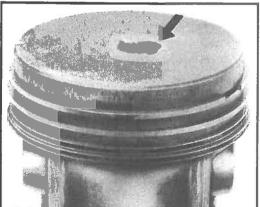
A noticeable knocking occurs when fuel in the cylinder ignites too early, too rapidly, or unevenly. The resulting "knock" can burn the piston, wear out the top groove, or cause the ring to break or stick.
