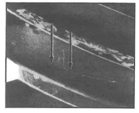
The initial appearance of case crushing of a carburized gear (a gear hardened by heating the surface, converting it to high-carbon steel, then quenching) is shown at the left and the final stages at the right.
