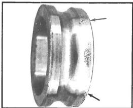
Foreign material caused excessive wear to these bearings. The roller ends are worn down to the indent and the ribs are badly worn.
