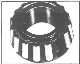
Fatigue damage was from an impact during either handling or mounting. An impact leaves a depression that can initiate premature fatigue.
