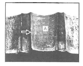
Another fatigue fracture is shown. The arrow indicates the crack origin at the left edge of the fracture, where a small pit existed near the base of the contact area on the pressure side of the tooth. The area just beside the crack origin (at arrow) is well rubbed, which indicates that the crack progressed slowly at first.
