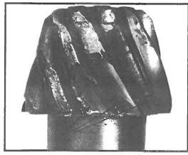
This gear failed from fatigue with severe tooth wear. The fracture extends from root fillets (the area connecting the bases of the teeth) to the bore in the gear.
