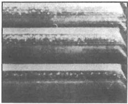
Destructive scoring is shown. Heavy scoring occurred above and below the pitch line. Usually, the damage progresses quickly and the gear fails.
