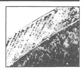
They start along the line of contact where the pressure in heaviest against the teeth of the mating parts and are generally caused by excessive loads. Frequently a fatigue crack will start at a pitted area. Spalls are an advanced state or severe form of pitting and part of the gear may crack off.
