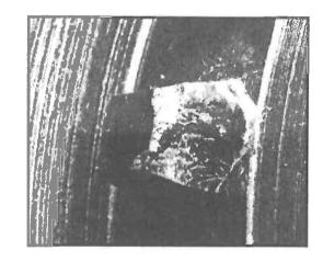
The break in the hardened spur gear has a gray, grainy appearance typical of the shock failure. It does not have the smooth appearance characteristic of fatigue. The failure probably resulted from improper clutching or improper shifting.
