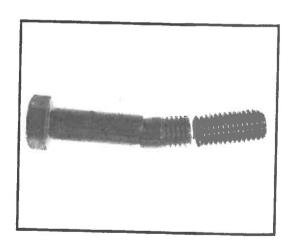
When friction is low, the recommended torque will produce too much tension on the bolt and cause this failure. Replace and reduce torque.
