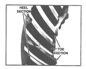
The fracture resulted from excessive loading on the toe section of the gear, while the cause of failure was insufficient backlash.
