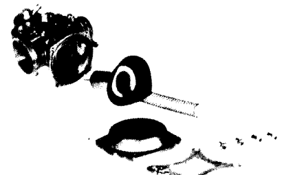
Carburetor top and throttle slide assembly
