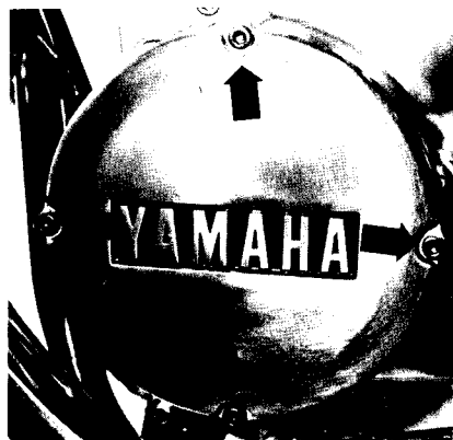
Alternator rotor cover allen bolts
