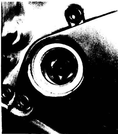
Clutch adjuster screw and locknut
