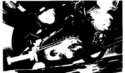
Chain adjusting bolt and swing arm alignment marks
