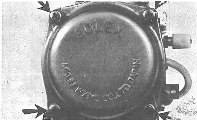
Cover securing screws
